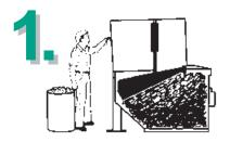
Operator inserts key and turns to "UP" position. When ram moves to up position the door can be opened.
