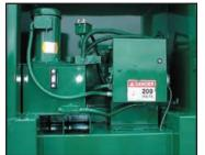
The side mounted power unit offers easy access for maintenance on the motor and electrical panel.
