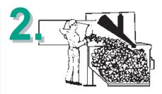
The large door opening allows even a 30 gallon container to be emptied easily. The new waste material is dumped into the cavity left in the container by previous ram position.
