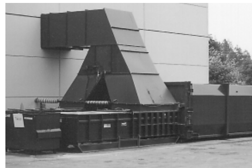
This manufacturing facility utilizes a conveyor and a custom chute system to feed two, RJ-575HD Compactors with reinforced compaction containers.
