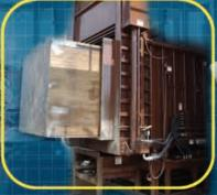
The BlokPak has a 5 ft. ram penetration. This ejects the final log into the trailer with very little spillage.
