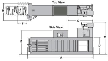
*Material Thickness:* Ram Face: 3/8" PL with 1" bars (1/4" PL on 620-E models; Ram Bottom, Bottom Liner, Ram Top, Floor, Floor Liner, and Charge Chamber Side: 3/8"; Bale Chamber Sides 1/4".
