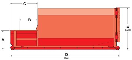
**Dimensions not shown:**  $8' - 4 \frac{1}{8}" (2543 \text{mm})$  Overall Width **Ground Roller Widths:**  $61 \frac{7}{8}" (1572 \text{mm})$  Inside Rollers
